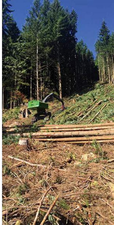
John Deere harvesting equipment at work using the Remote Operated Bulldozer (ROB) winch assist system, at the Demo 2016 show.
