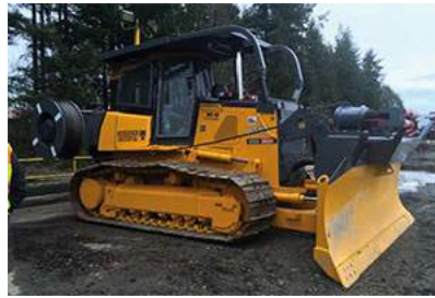
John Deere dealer Brandt Tractor and Island Pacific Equipment outfitted Clusko with a John Deere 850J ROB with a two-winch system attached. The winches are powered by the 850J's hydrostatic drive motors
