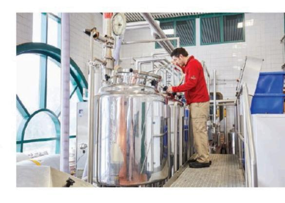
The pilot brewery has vessels that mimic larger vessels in the other breweries so small batches can be made with new ingredients and processes.
